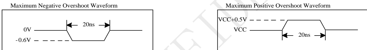
Figure 5-1 Maximum Overshoot Waveform
